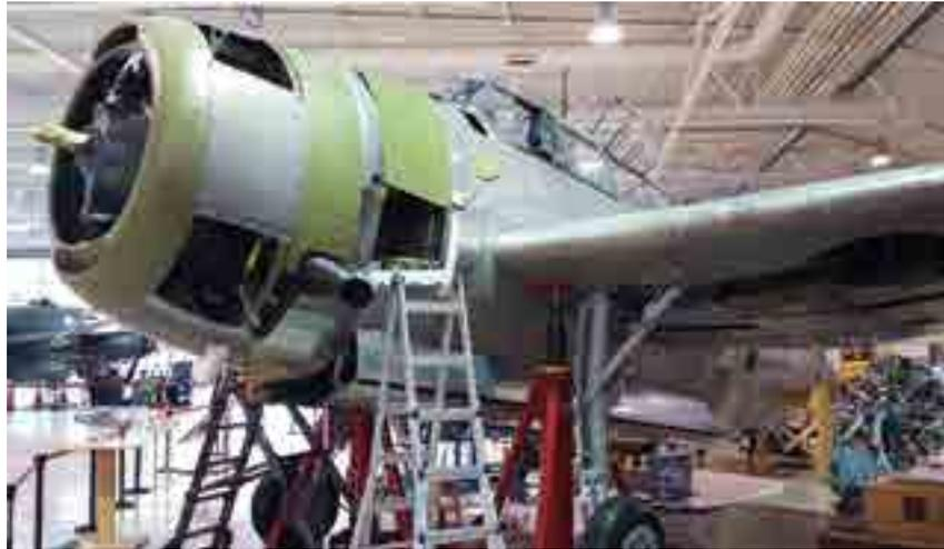
CWH's Avenger on the aircraft jacks for the landing gear swings and testing. The aircraft has now been removed from the jacks, the wings have been folded and restoration continues towards its completion to flying status. AL MICKELLOFF
