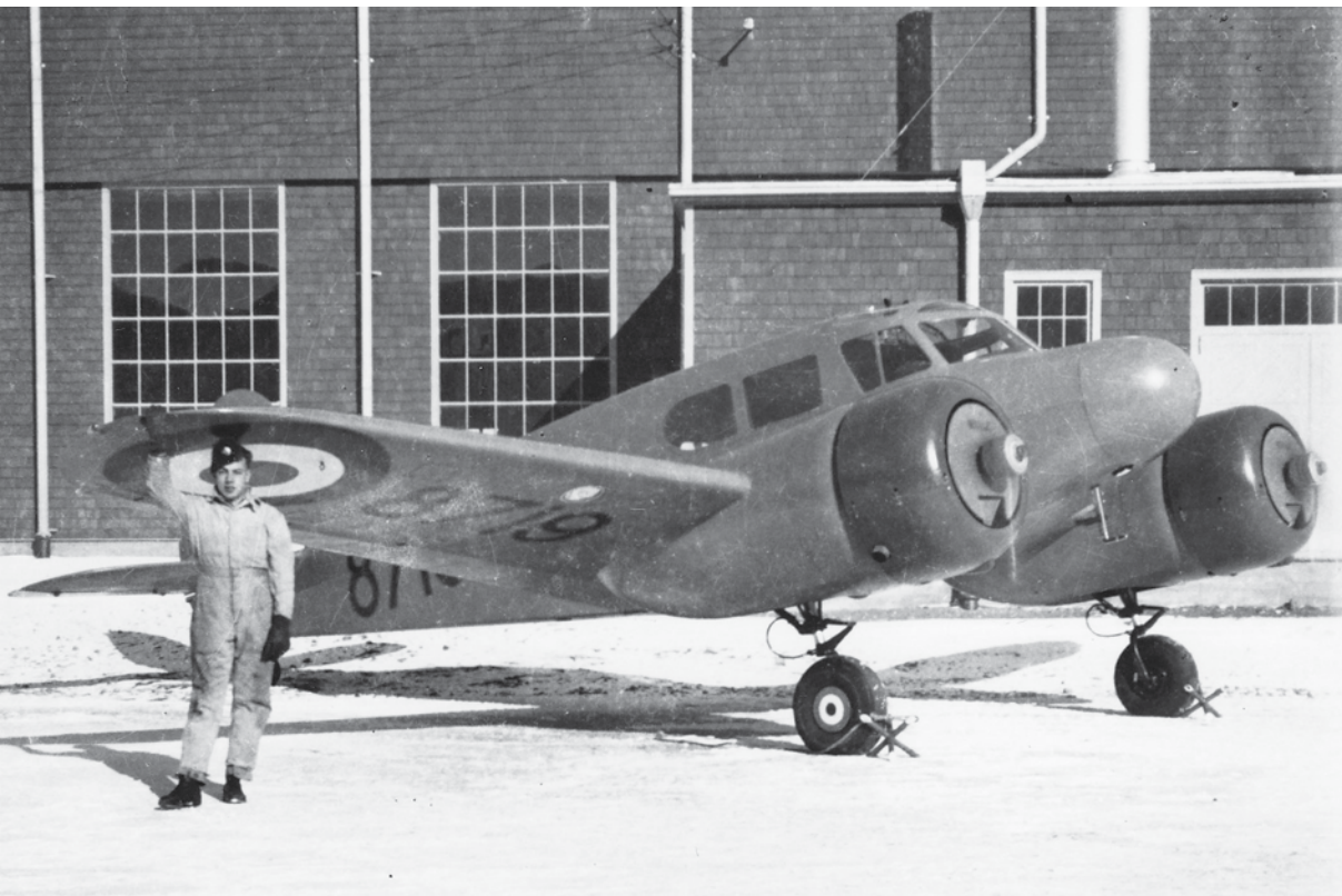
Crane #8719 of No. 15 SFTS, Claresholm, Alberta. Note the engine covers used during winter operations and the different colour engine cowl. The young airman in the photo is unknown. JACK MCNULTY COLLECTION VIA GORD MCNULTY
