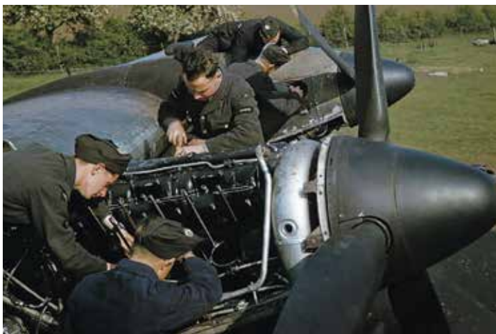
Fitters servicing the port Mk. XX Merlin engines of a 35 Squadron Halifax Mk. II in the summer of 1942. The large coolant header tank of the port inner engine is clearly visible. IMPERIAL WAR MUSEUM
