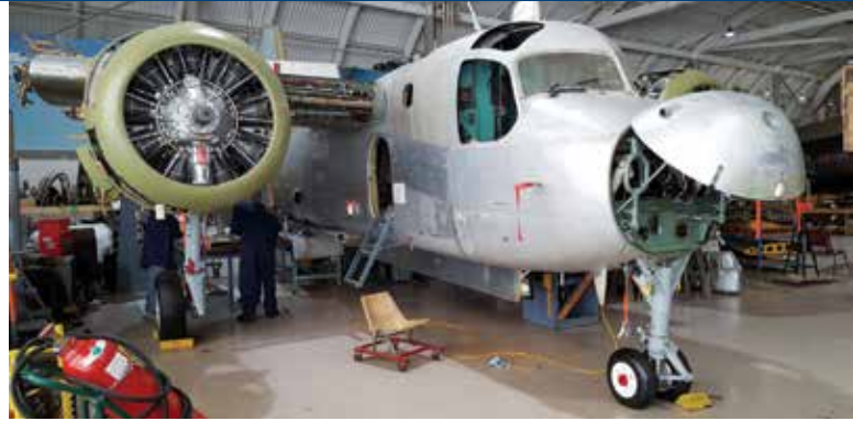
Tracker restoration progress to date, showing the installation of the nose gear. AL MICKELLOFF
