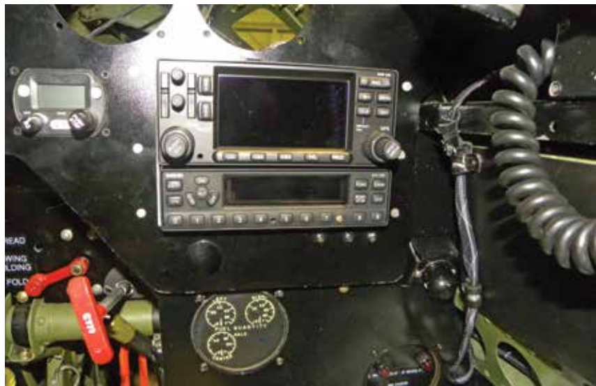
Work is proceeding well on the front cockpit instrument panel, showing the installation of the new GPS and radios. DON COIT
