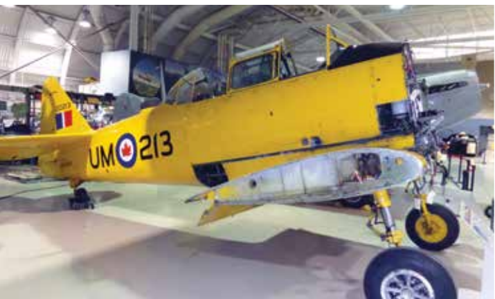
Harvard CF-UUU minus its wings and engine undergoing a full inspection. BILL CUMMING
