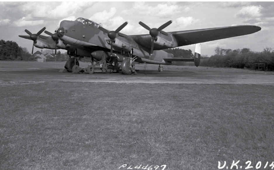
A 617 Squadron Lancaster being loaded with a Tall Boy bomb. Note the absence of the nose gunner turret. DND
