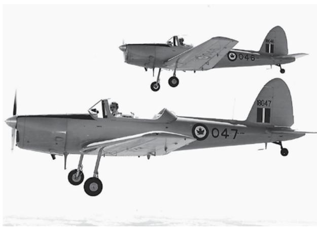
Two RCAF Chipmunks (18046 & 18047) over north Toronto prior to delivery to the RCAF. Note the bubble type canopy as specified by the RCAF. DE HAVILLAND CANADA
