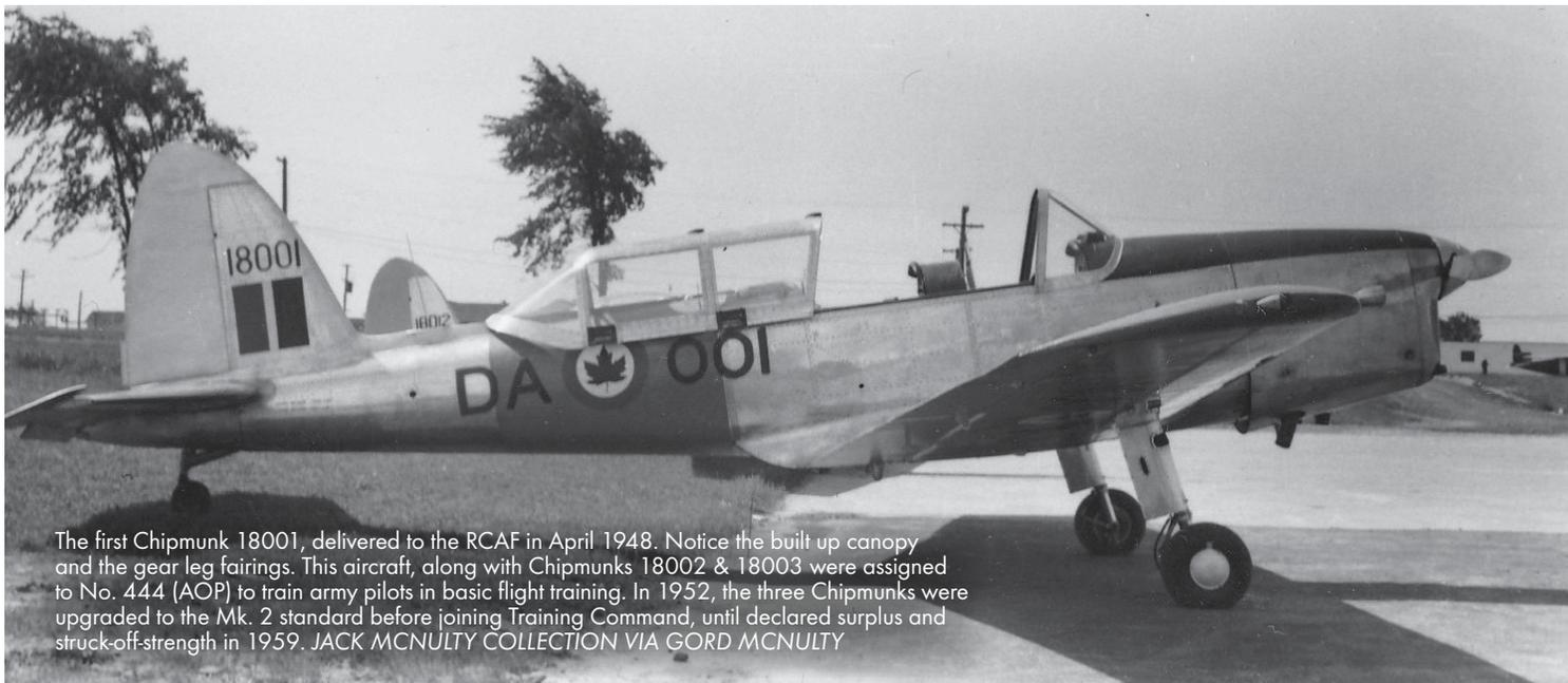
The first Chipmunk 18001, delivered to the RCAF in April 1948. Notice the built up canopy and the gear leg fairings. This aircraft, along with Chipmunks 18002 & 18003 were assigned to No. 444 (AOP) to train army pilots in basic flight training. In 1952, the three Chipmunks were upgraded to the Mk. 2 standard before joining Training Command, until declared surplus and struck-off-strength in 1959. JACK MCNULTY COLLECTION VIA GORD MCNULTY
