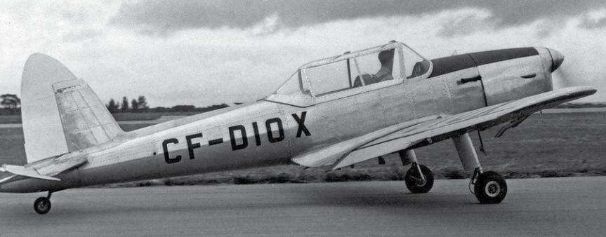
The prototype DHC-1 Chipmunk at Downsview about 1948. Notice the built up Perspex canopy, as provided with the first few Canadian built Chipmunks.
