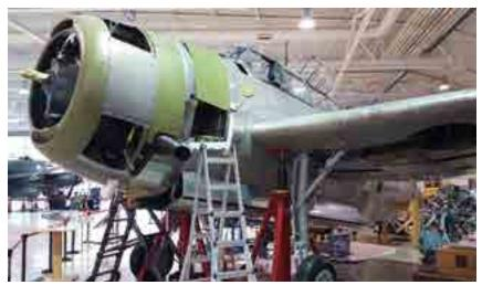
CWH's Avenger on the aircraft jacks for the landing gear swings and testing. The aircraft has now been removed from the jacks, the wings have been folded and restoration continues towards its completion to flying status. AL MICKELOFF
